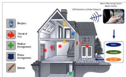
Intruder Alarm System
